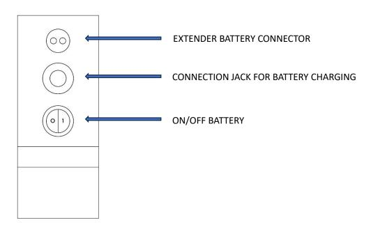
If a connector is accidentally disconnected during opening and closing operations, the display may not turn on. In that case, simply turn off and turn on the battery to reset the system.
