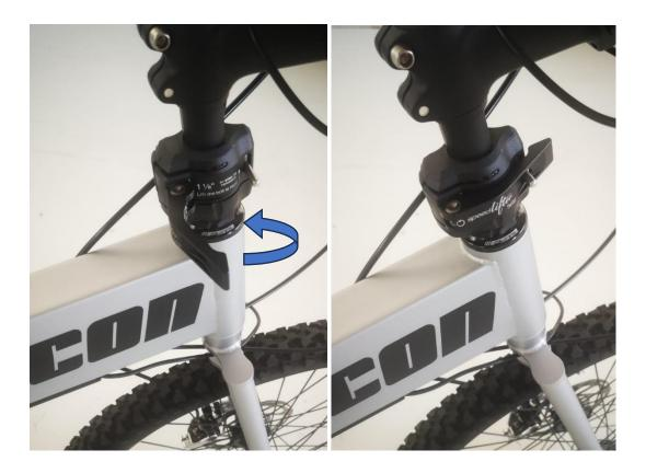
You are ready to unfolding the bike. You can do it with a strong blow by detaching the magnets that hold the frame together. Holding the left hand steady, bring the right hand back by pulling the seat back and making it rotate upwards in order to bring it back to the rear wheel. Tilt the bike on the wheel by pivoting on the front wheel facilitates this operation especially if you completely detach the front wheel from the ground.
