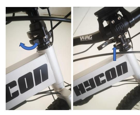
To rotate it, lift up the small lever, rotate it until it is in front of you in the forward position, you will hear a 90° click, tighten the lever. Hold the handlebar with your left hand and pull the front brake to stop the wheel.
